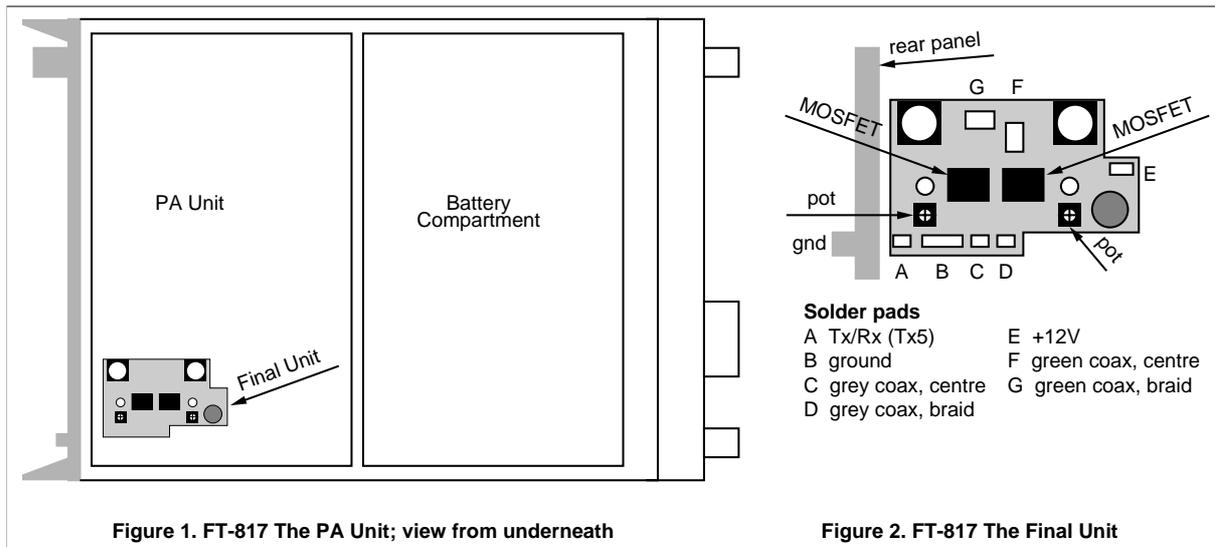
Remove the screw located in the centre of the lower cover by the edge of the battery compartment and then remove the 5 screws around the edge of the cover. Gently prise the cover away from the chassis.
