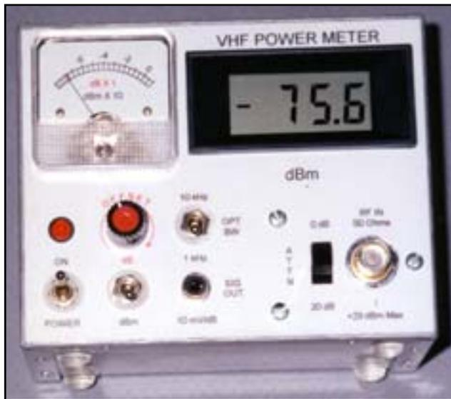
**Fig 1**—The advanced VHF power meter includes a digital panel meter for accurate, high-resolution power readings plus an analog meter for trend information. The instrument bottoms out around -76 dBm but calibration very good above -70 dBm.
