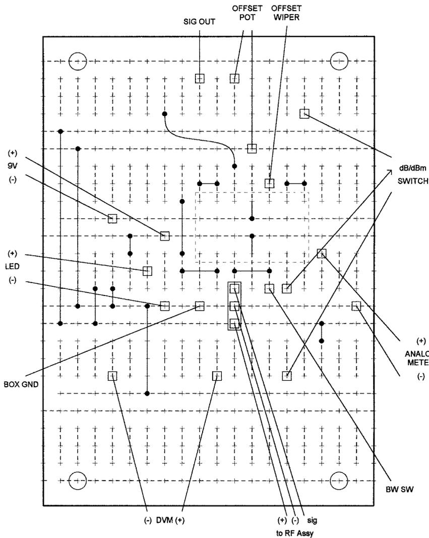
**Fig 7—**Wiring and jumper diagram for the signal-processing board. This view is from the component side with the printed-circuit traces and lands from the other side shown dotted.
