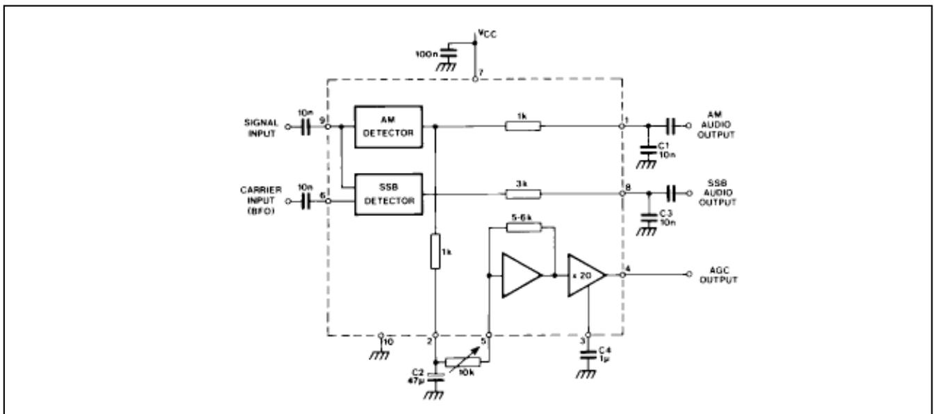
Fig.2 Block diagram
