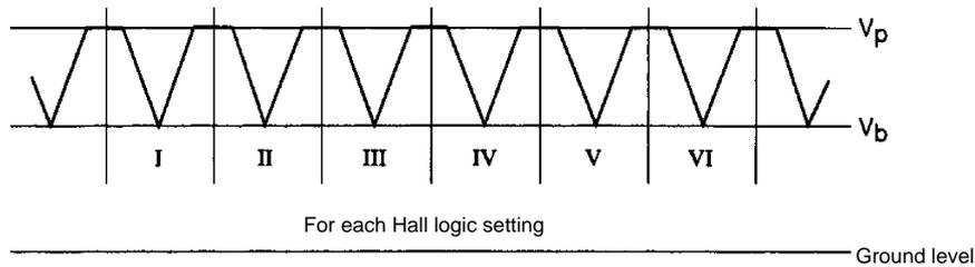
$$\text{Correction ratio} = \frac{2 \times (V_p - V_b)}{V_p - V_b} 100 \times (\%)$$
