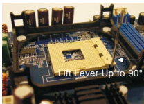
STEP 1: Lift The Socket Lever Up to 90°
