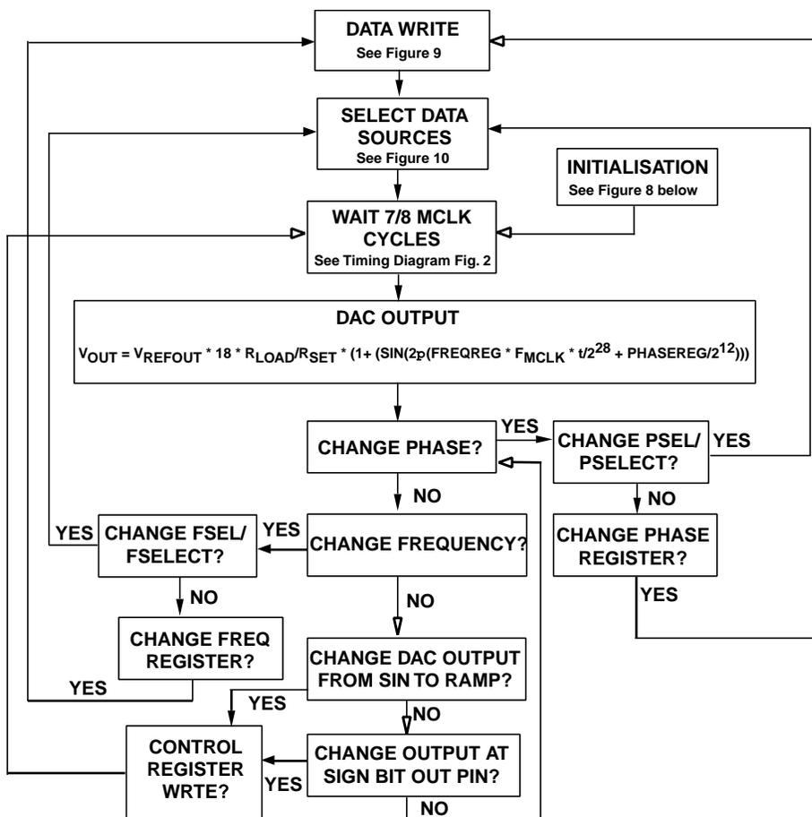
Figure 7. Flow Chart for AD9834 Initialisation and Operation
