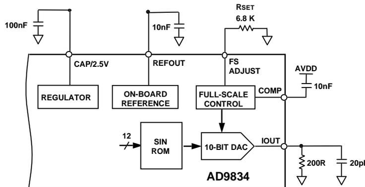
Figure 1. Test Circuit With which Specifications are tested.
