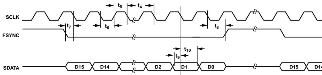
Figure 3. Serial Timing
