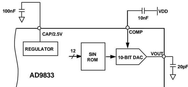
Figure 1. Test Circuit With which Specifications are tested.
