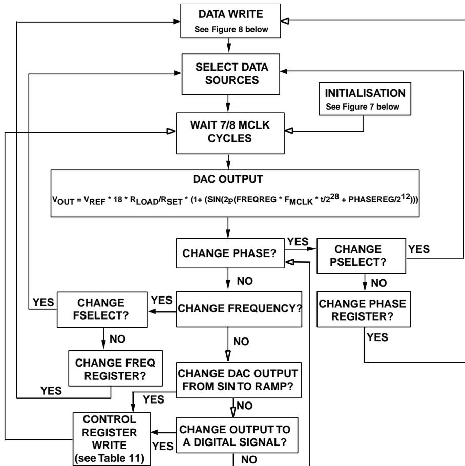
Figure 6. Flow Chart for AD9833 Initialisation and Operation
